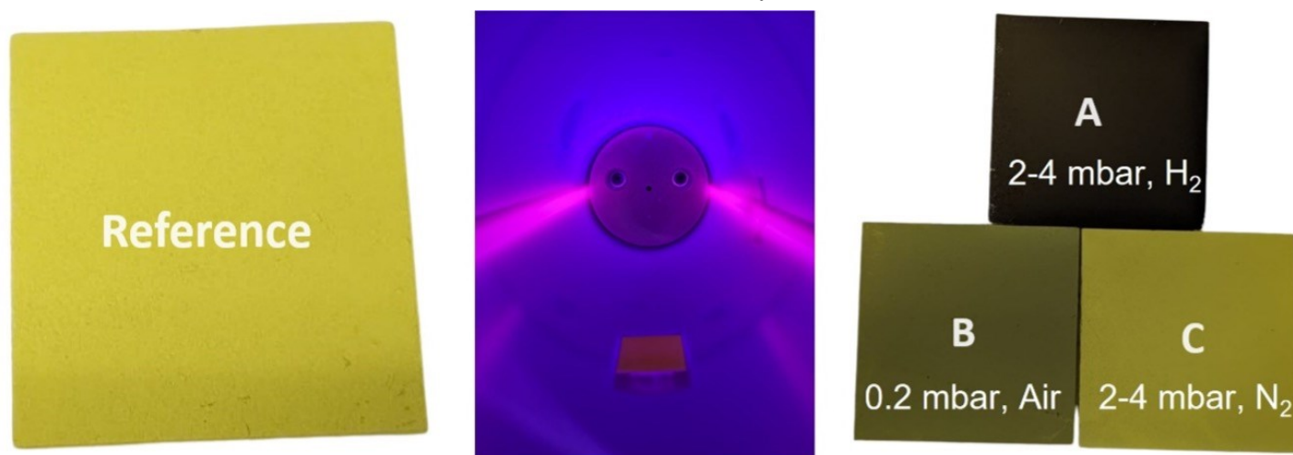
Figure 1: Schematic illustration of pristine and plasma treated BiVO 4 spray coated on a pre-cleaned glass substrate. Plasma treatments were performed in a Diener Zepto low-pressure plasma chamber at 100 W using the gas atmospheres indicated above.
